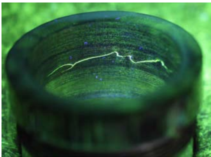
图 8 桨轴内圆面裂纹形貌荧光检查 Fig. 8 Fluorescence inspection of crack morphology in the inner surface of the propeller shaft
